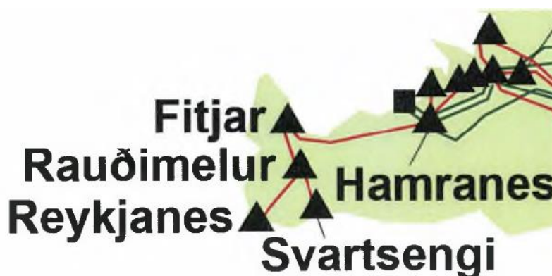
Figure 2. Connection of Fitjar substation to the main grid. The 220 kV grid is shown in green and the 132 kV grid is shown in red.
