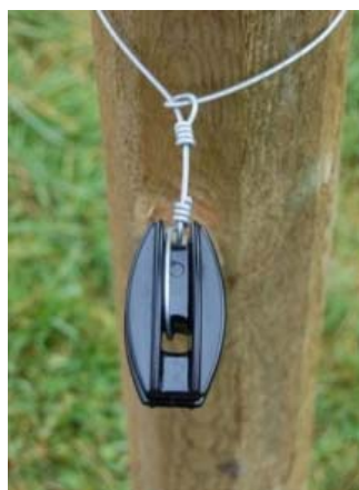
Figure 3. Specialised insulators must be used where there are sharp angles in fence direction. (Photo: DeLaval/ Jan Pettersson).
